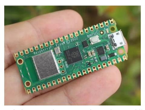
As you can see it looks very similar to a normal Pico, the main difference is the metal enclosure towards the left-hand end of the board - this houses the electronics for the WiFi and at the extreme edge of the board is the trapezoidal antenna.
